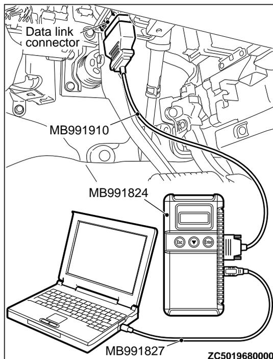
**STEP 2. Using scan tool MB991958, read the audio diagnostic trouble code**
