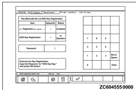
4. Enter the password for keyless operation key registration and press the OK button. Then the keyless operation key registration starts.
