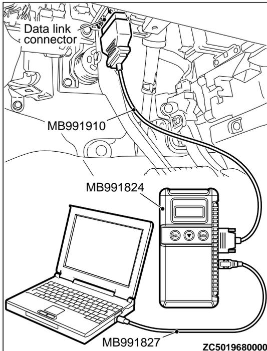
**STEP 3. Using scan tool MB991958, read the actuator test.**
