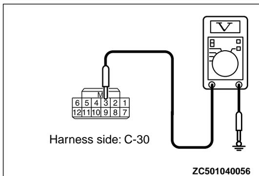
**STEP 11. Using the oscilloscope, check the waveform at receiver antenna module connector C-30 and ground by backprobing.**
