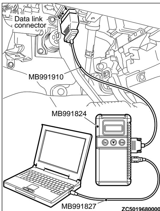
**STEP 2. Check the VIN registered in the engine control module and the vehicle's VIN.**
