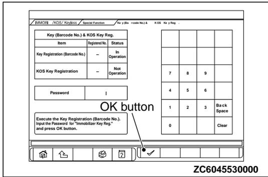
1. When "Key(Barcode No.) & KOS key Registration" screen is displayed, enter the password for the key registration and press the OK button.
