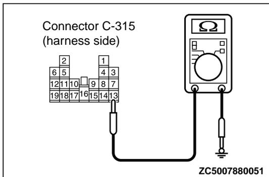
**INSPECTION PROCEDURE 7: Driver's Door Lock Switch does not Work.**
