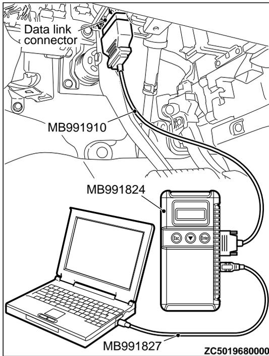
**STEP 2. Register the keyless operation key ID and recheck the diagnostic trouble code.**
