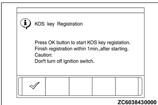
2. When the key registration is completed, "Completed." is displayed. To continue the key registration, press the OK button according to the screen instructions. Then "Executing!" is displayed again and the next registration process starts. To finish the key registration and start the keyless
