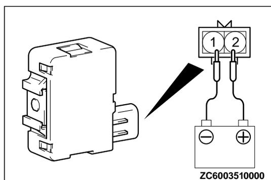
(2) Check that the outer tone alarm sounds once when the terminals are connected to the battery as shown.
