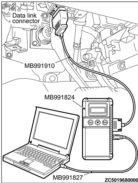
**STEP 1. Using scan tool MB991958, diagnose the CAN bus line.**
