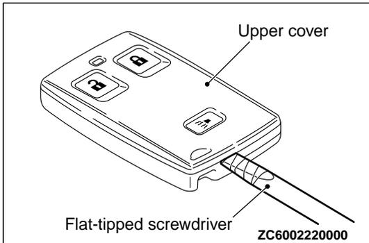
**ASSEMBLY SERVICE POINT****>>A<< BATTERY INSTALLATION**
