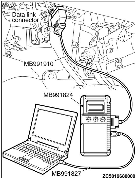
**STEP 2. Using scan tool MB991958, read the A/C diagnostic trouble code**
