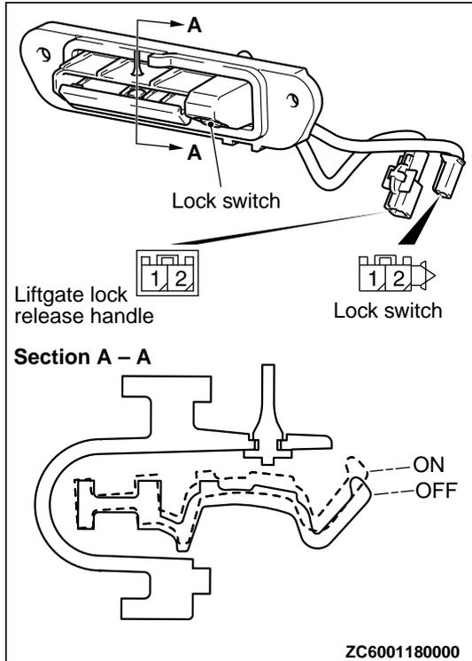
terminals pushed back in the connector. Repair the wiring harness as necessary. Check that the liftgate lock release handle works normally.
