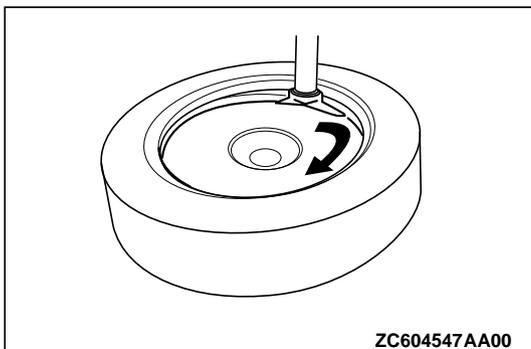
2. Engage the shoe and make sure that 20 cm (7.9 inch) is maintained between the cross point and the valve. The arrow shows the direction of rotation of the wheel.
