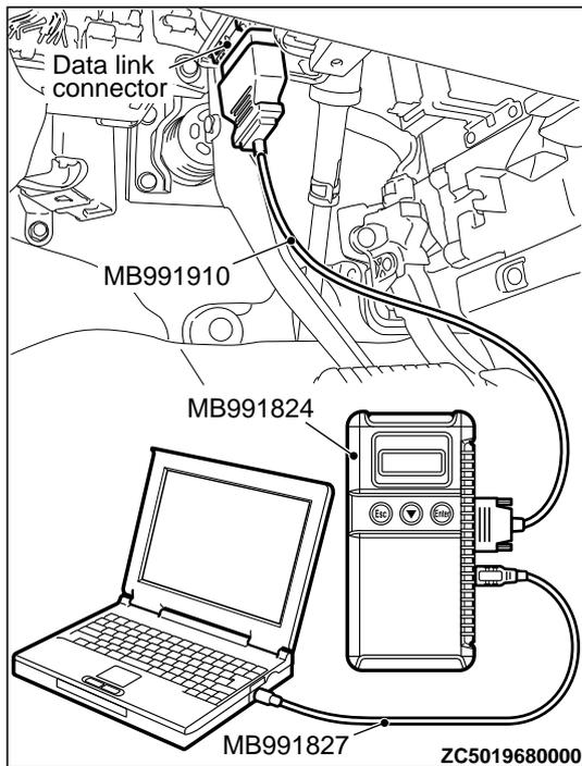
**STEP 1. Using scan tool MB991958, read CAN bus the diagnostic trouble code.**
