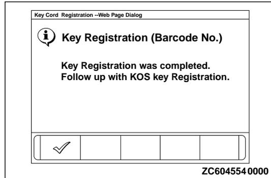
3. "Key Registration was completed. Follow up with KOS key Registration. " is displayed, press the OK button and go to the keyless operation key registration.
