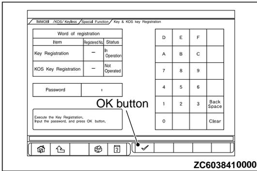
1. When "Key & KOS Key Registration" screen is displayed, enter the password for the key registration and press the OK button. Then, "Executing!" is displayed and the key registration process starts.
