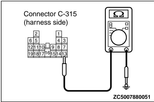
(3) Check for continuity between the C-315 ETACS-ECU connector terminal No. 13 and the ground.
