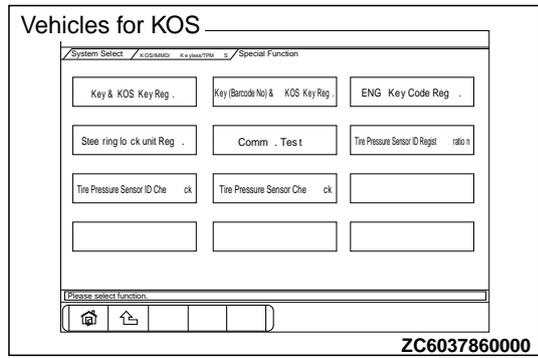
4. Select the button of the operation to be performed from the "Special Function" screen.
