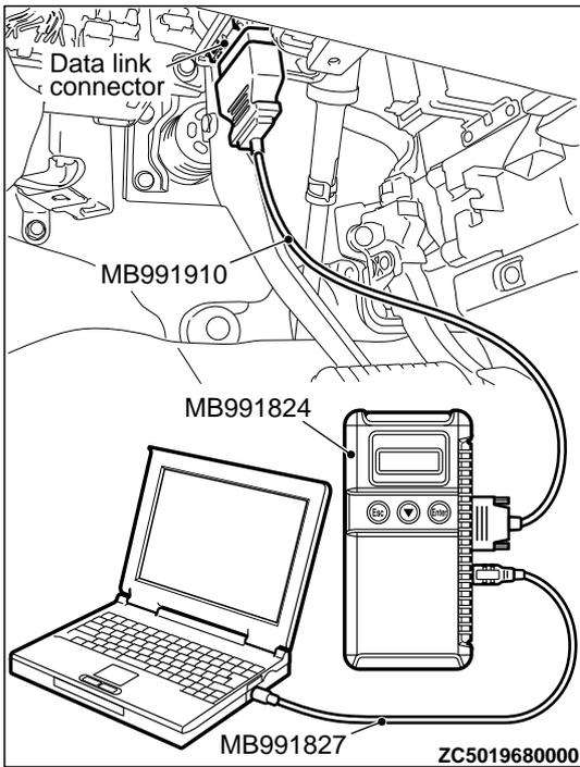
Connect the M.U.T.-III to the 16-pin data link connector as follows.
