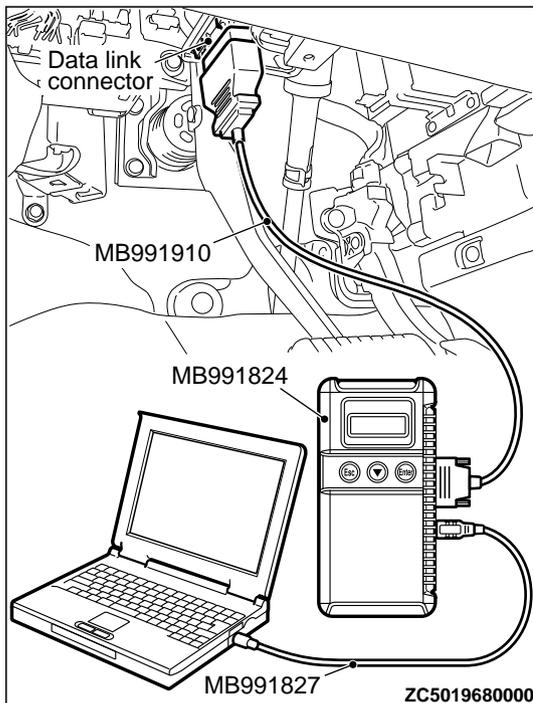
**STEP 3. Using scan tool MB991958, Check the configuration function.**
