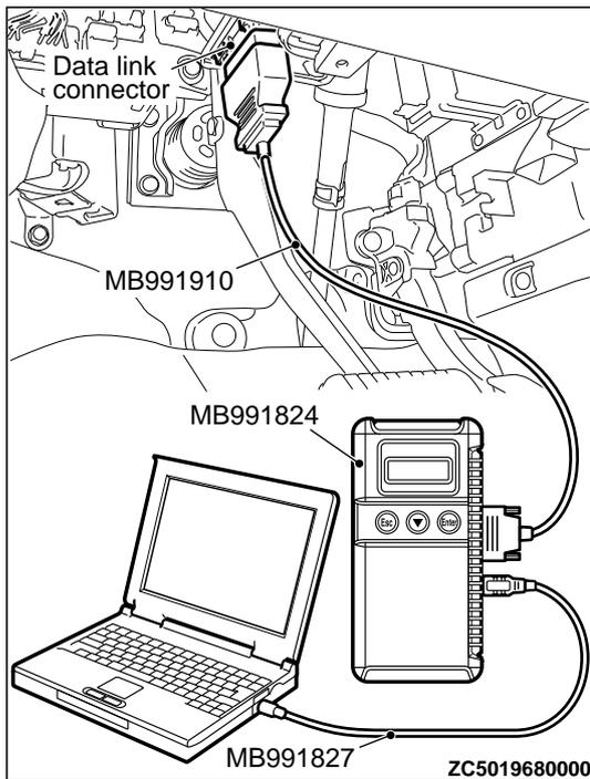
**STEP 1. Using scan tool MB991958, read the diagnostic trouble code.**
