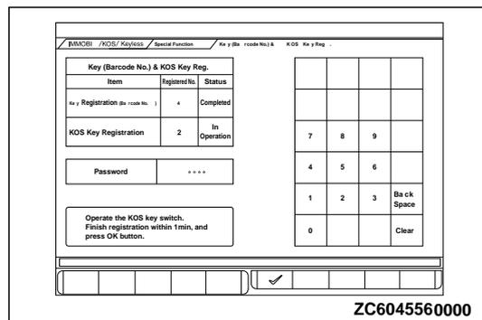
5. Press the lock switch of the keyless operation key to be registered twice within 1 minute to allow the keyless operation key to be registered. Complete the registration within 1 minute and press the OK button. Then the keyless operation key registration ends.
