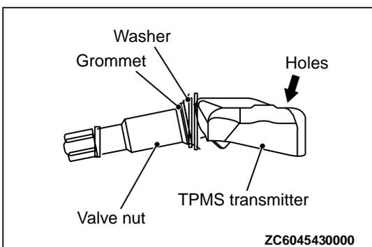
2. Mount TPMS transmitter valve through rim hole as illustrated. Pressure holes in the transmitter case should face away from center of rim. Tighten valve nut finger tight, then slowly torque the valve nut to  $8.0 \pm 0.5$  N·m ( $71 \pm 4$  in-lb).
