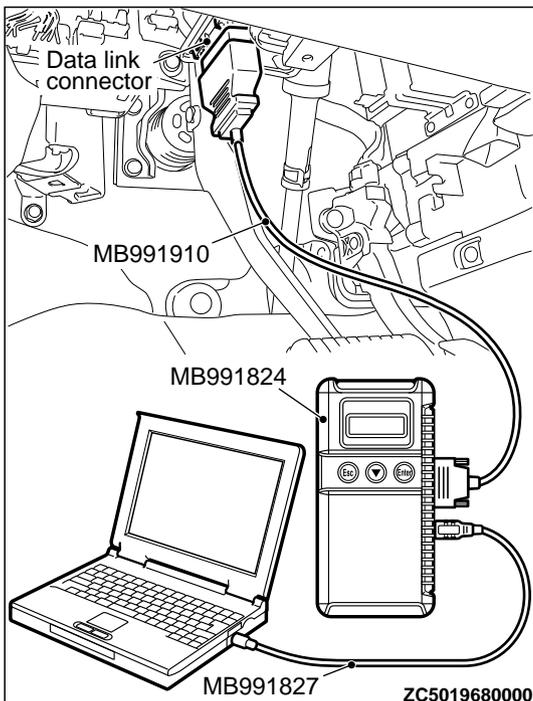
**STEP 2. Using scan tool MB991958, read the diagnostic trouble code.**
