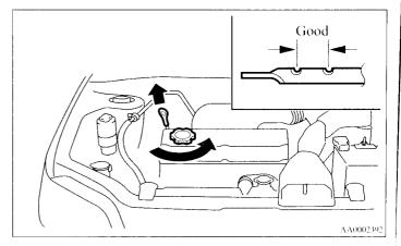
Overfilling the crankcase will cause oil aeration and loss of oil pressure, which could damage the engine.
