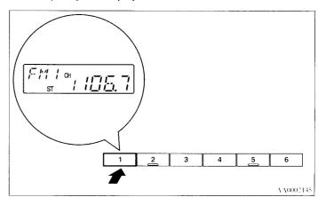
3. The preset memory setting is retrieved by pressing the button and then releasing it within about 2 seconds.
