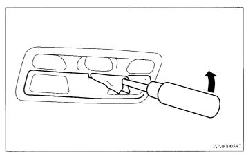
Insert a screwdriver into the notch of the light assembly. Pry gently to remove the lens, then remove the bulb from the light holder.
