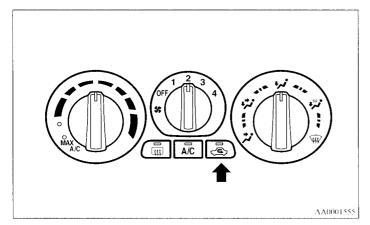
If the outside air is dusty or contaminated in some way, use the recirculation position. Switch to the outside position every now and then to keep the windows from fogging up.
