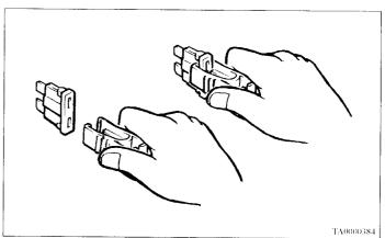
6. Use the fuse location diagrams and the matching tables, to check the fuse that is related to the problem. If the fuse is not blown, something else must be causing the problem. Contact an authorized Mitsubishi dealer to have the problem checked.
