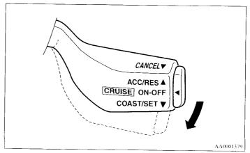
To slow down in small amounts, press the cruise control lever down for less than 1 second and release it.
