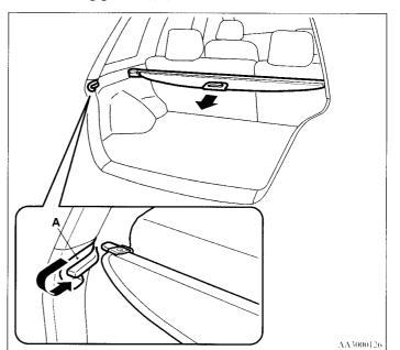
2. Remove the cover from the mounting grooves, and the cover will be rolled back into the retracted position.
