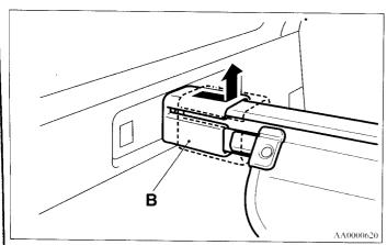
To fit the tonneau cover, follow the removal steps in reverse. Gently shake the entire tonneau cover after fitting it to make sure it is securely retained.
