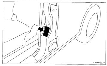
The recommended inflation pressures should be used for the tires listed below.
