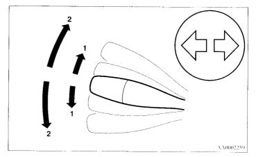
If this light flashes faster than usual, check for a burned out lamp bulb or faulty connection in the signal.
