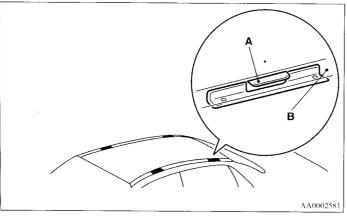
When installing the roof carrier, use the brackets (A). The brackets are located under each roof drip moulding (B).
