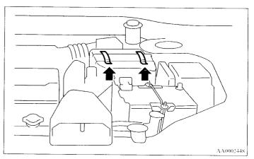
After replacing the air cleaner filter, put the cover (resonator) back on in its original position.
