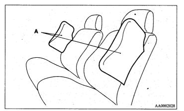
A label is attached to the seat backs in vehicles with side air bags.
