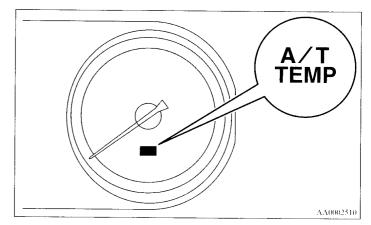
If the light comes on, reduce the engine speed and stop the vehicle in a safe area. Then set the selector lever to "P" (PARK) position and idle the engine until the warning light goes off. When the warning light goes off, resume normal driving. If the warning light does not go off, have your vehicle inspected at an authorized Mitsubishi dealer.
