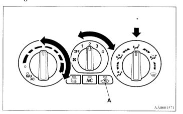
Set the mode selection dial to the "•••" position and set the air selection switch (A) to the outside position.
