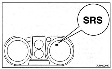
When the ignition key is turned to the "ON" or "START" position, the warning light should come on for several seconds and then go out. This means the system is working properly. The SRS warning light is shared by the driver's air bag, the front passenger's air bag, the optional side air bags, and the seat belt pre-tensioner.
