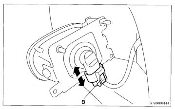
Remove the entire socket and bulb assembly (C) by turning it counterclockwise.
