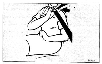
3. Pull the seat belt out slowly while holding the metal tongue. The belt will not lock if you stop or hesitate, so relax and continue to "buckle-up".
