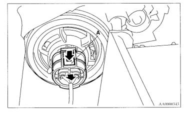
Remove the locking cap (B) by turning it counterclockwise.
