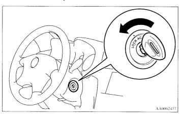
First set the selector lever to the "P" (PARK) position, and then turn the key to the "LOCK" position and remove it.
