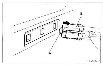
2. After changing the position, gently shake the entire tonneau cover to make sure it is securely retained.
