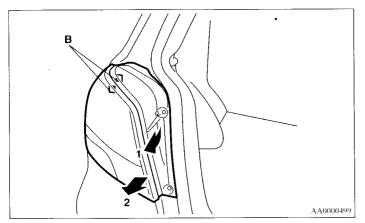
After remove the socket and bulb assemblies by turning them counterclockwise, remove the bulb by pulling it out.
