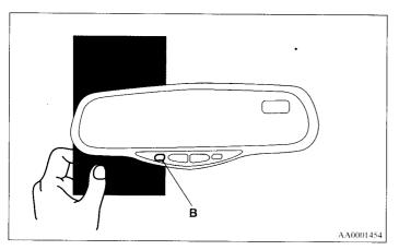
2. While in a well-lit area, make sure light strikes the sensor on the front of the mirror, simulating glare from vehicles behind you.
