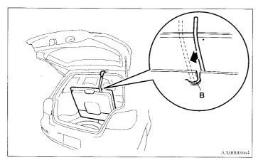
3. To remove the spare tire, remove the installation bolt with the wheel nut wrench (C) by turning it counterclockwise.
