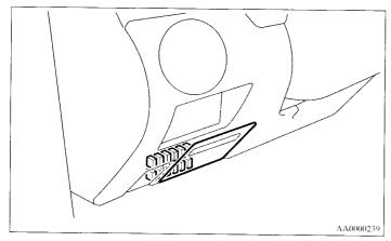
The fuse block in the passenger compartment is located behind the personal box.
