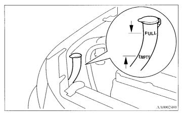
When freezing weather is anticipated, flush out the water in the reservoir by operating the pump. Fill the reservoir with windshield antifreeze (not radiator antifreeze), and operate the system for a few seconds to flush out the residual water.
