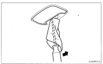
Insert a screwdriver into the notch of the light assembly and pry gently to remove the lens. Pull the light bulb out from the light holder.
