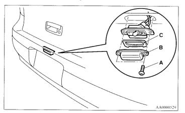
Remove the socket and bulb assembly together by turning it counterclockwise, and then remove the bulb by pulling out.
