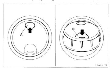
Change the direction of the airflow by turning the vents itself.
