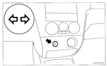
If you press the flasher switch, the front and rear turn signals will flash intermittently, and so will the hazard warning lights. This is an emergency warning system and should not be used when the vehicle is in motion, except for emergencies.
