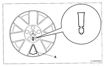
Line up the wheel nuts with the wheel cover mounting holes, and line up the air valve with the valve opening (A) on the wheel cover.
