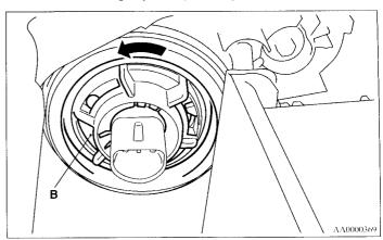
Remove the headlight bulb (C) with holder.
